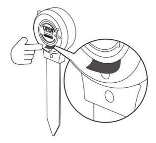
1. RemOve the insulating sheet when first used.
