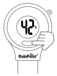
2. Insert it into the soil until the soil reach the "BEST" line and press the button. The data will display after 3 seconds.
