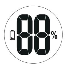
When the device has low battery, a low battery prompt will be displayed on the screen, reminding you to replace the battery.
