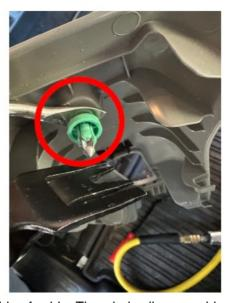
• Gently wiggle and pry towards inside of cabin. The whole clip assembly and cover can remove together:
