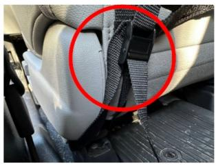
Tighten the top straps as desired while maintaining desired range of motion for the front seats. Finally draw the bottom straps tight just enough to not pull down the net past desired height position. Cover up the buckles and wrap up excess adjusting strap:
