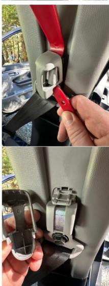
• Remove the exposed 14mm bolt securing the upper seat belt adjuster:
