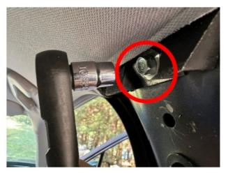
• Slide the C100G hardware piece supplied with your net onto this bolt. Reinstall and finger tighten to start the threads and then twist the tether and D ring oriented to the top:
