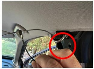
• Put the metal part of the clip back into the channel location and realign so that the whole cover will line up correctly:
