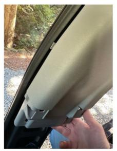
The service manual says that this clip should be considered a "one use" clip and to use a rubber mallet and a towel to tap it in, breaking off the profusion tabs.
