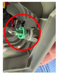
• Slide the whole clip assembly down and out of the upper panel cover.
