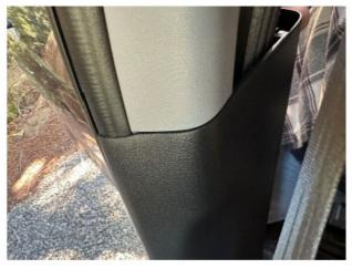
• Press the lower panel into place ensuring that all tabs line up correctly.
