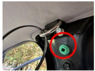
Remove the clip from the previous step by sliding down and off of the trim cover. You can then lift the side tabs of the green piece from the metal insert and reinstall the green receptor back into the B pillar opening hole:
