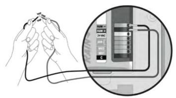
2. If the controller appears to be working, while the sensor is still disconnected measure the open circuit voltage on the controller's sensor input terminals. This voltage must be between 8...24V DC for the sensor to operate.
