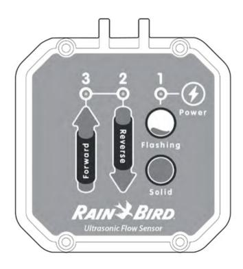
Under standard operation, water flowing forwards through the system; indicator light 1 should be solid on, indicator light 2 should be off and light 3 should be flashing. Other indicator states are described on the following page.
