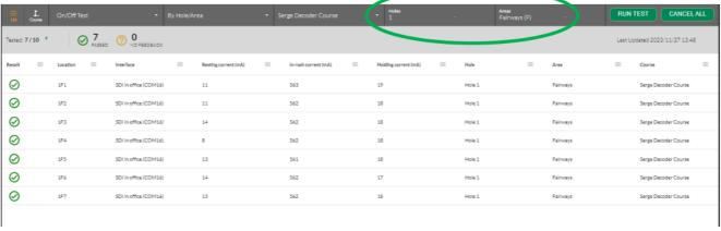
Results are displayed in a table showing the different current values at each step (Resting, In-Rush and Holding).
