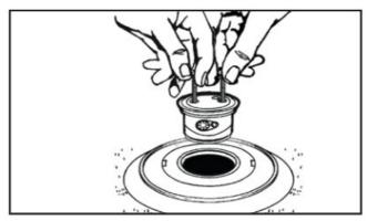
3. Press the replacement nozzle assembly into the nozzle housing, making sure the nozzle front is flush with the outside of the housing.
