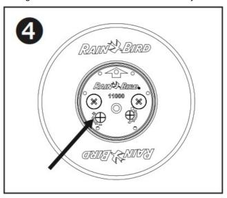
**CAUTION:** Turning the arc adjustment past the stop may damage the internal.
