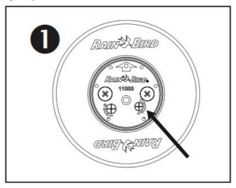
**IMPORTANT NOTE:** Apply downward pressure on screw driver to ensure it fully engages into the slot.
