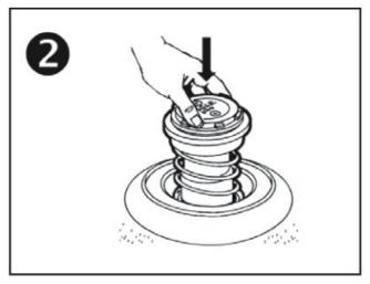
3. Clean and position the snap ring in the groove on the top of the rotor case with the bottom of the snap ring facing down.
