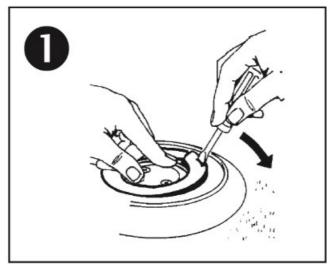
NOTE: You MUST press down on the nozzle housing when removing the snap ring.
