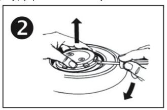
3. Lift the internal assembly up and out of the case.
