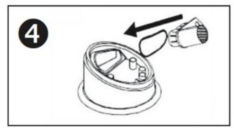
**CAUTION:** If the nozzle is not flush and seated properly in the nozzle housing, the rotor may not perform properly.
