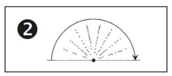
3. For best results, turn the head ON to see where both legs "trip" (the trip point is the point where the rotor turns and begins rotating in the opposite direction). To manually advance the nozzle housing, SLOWLY move it in the same direction it is currently moving. After noting where the head trips, return the head to the left trip point. CAUTION: Do not turn the turret manually against the direction of rotation while in operation.
