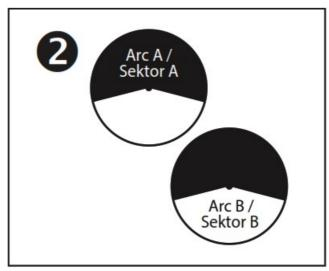
**Note:** When internal is removed from the case, to ensure the rotor is in the Primary arc, put internal in Full Circle align arrows on riser assembly and nozzle base, then put the unit back into Part Circle mode. Install the internal in case.
