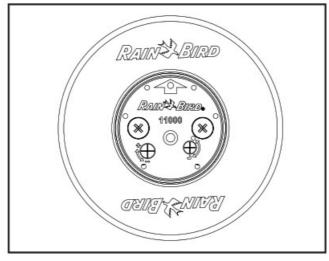
2. The RIGHT leg of the arc is the adjustable leg. It is shipped from the factory at approximately 180 degrees from the fixed leg.
