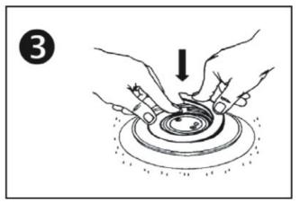
Press the end of the snap ring without the screwdriver slot into the groove. Press and twist the snap ring down in a circular motion until it is installed about two-thirds of the way.
