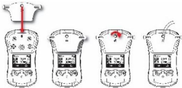
Install the calibration adapter on the QRAE 3 diffusion model
