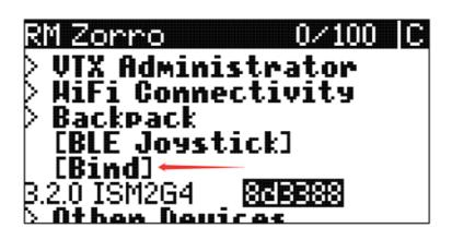
**Note:** To bind the receiver a second time or to another radio, power cycle the receiver 3 times. On the third power cycle, the LED will double blink, indicating bind mode. If you cannot successfully enter bind mode with the 3 power cycle method, you can hold down the boot button for 10 seconds to reset the receiver to bind mode or use the passphrase method below.
