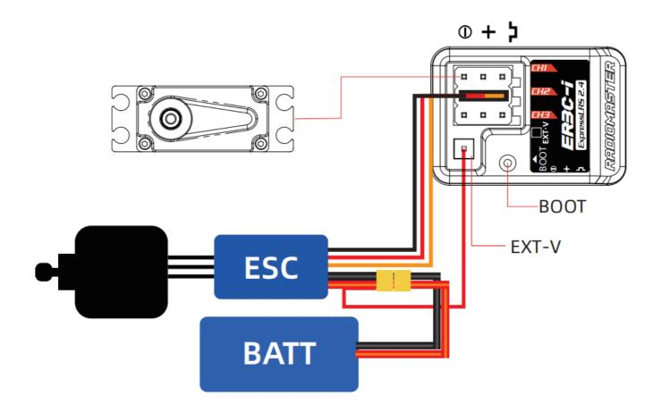
The Radiomaster ER3C-i ELRS receiver can drive three steering engines simultaneously. Integrated receiver voltage detection, power battery voltage detection, and realize the automatic switching of two voltage detection. With built-in antenna design, suitable for ship model, car model.
