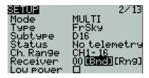
Long press the MDL button to enter the model settings, select MULTI in the SETUP page, and select the desired protocol in the sub-options. The system will automatically turn on the corresponding RF module according to the RF protocol you selected.
