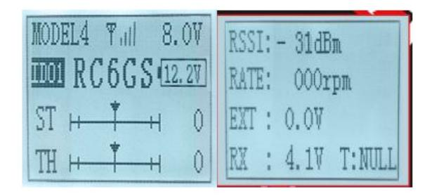
Warning can be set with a certain low RSSI value after testing by changing distance: Press EXIT and ENTER simultaneously to enter MENU=>press Inc(+) to highlight "19. ALARM =>Press ENTER to (dis)activate the warning and set the RSSI warning value.
