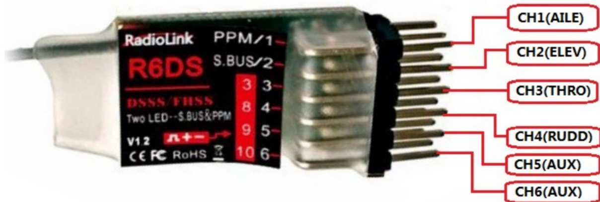
PWM signal working mode, 6channel
