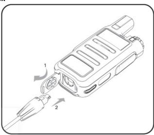
Installing the Speaker/Microphone
