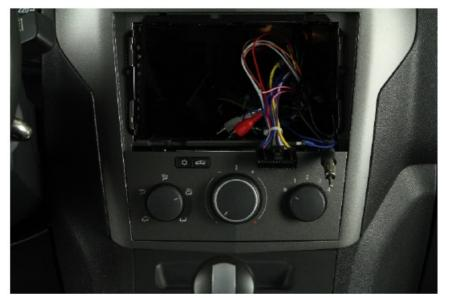
7. Neatly arrange the wires to the side, making room for the Radical device. Carefully slide it into the radio slot. Push back the R-C12OP2 until you hear the clicking sound of the latching mechanism. The installation of your R-C12OP2 is now complete.
