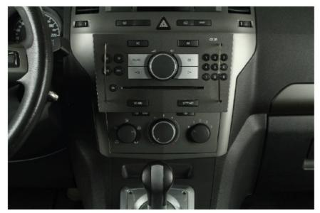
3. To completely remove the OE radio, all the cables (i.e. main wire harness, antenna cable etc.) must be unplugged on the backside of the device. Put the radio aside in a safe place, to protect it from damage.
