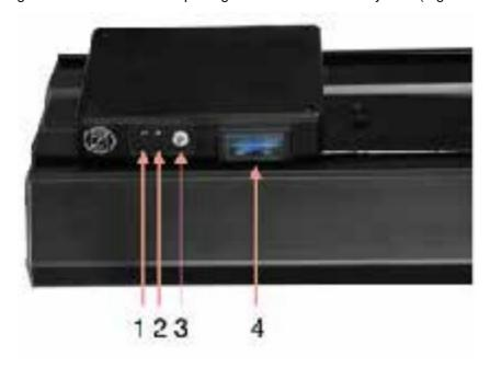
On the right see the drawing of the signal lights and button of Receiver01.
