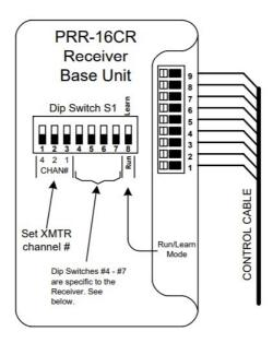
RSSI Indicator\* – The receiver has a Signal Strength Indicator to show the signal strength of the Transmitter. This is a test mode and can only be used during installation. See Diagnostics on page 20. Once the system is operational, set Switch #7 DOWN to turn off the RSSI.
