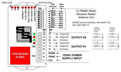
GENERAL – The PRR-16CR serves as a base unit, and termination point for the PRNR-1600C receiver radio/antenna unit. It contains a power supply, output relays and all connection points for the receiver/antenna unit.
