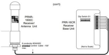
POWER INPUT – The PRNR-1600C receives its power supply from the PRR-16 Receiver Base unit.
