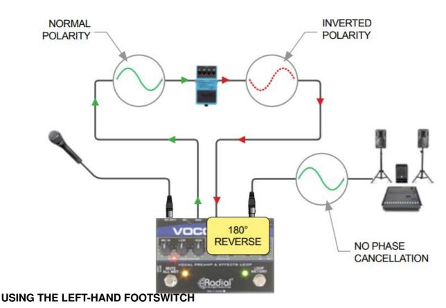
The left footswitch can be assigned as either a 'mute' switch or as an 'all-wet' effect loop. The function is selected using the recessed MUTE/LOOP switch on the left side. Use a small screw driver to change the position of the switch between inward and outward.
