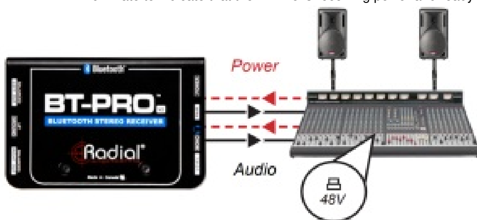
Powering the BT-Pro using 48V phantom power
