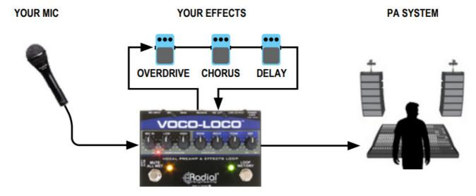
You simply prepare the effects in advance by turning on an echo and a chorus pedal and when ready, engage the pedal chain by depressing the effects loop footswitch. When the song is over, you stomp on the footswitch again to turn off the effects. In between songs you set up the next effect with your pedals on standby, ready to be engaged as needed.
