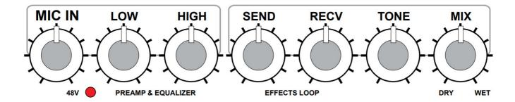
Turn on the PA system and slowly increase the level while speaking into your mic. Always test at low levels for safety. If you encounter buzz or hum, push in the recessed ground LIFT switch on the rear panel. This disconnects pin-1 on the XLR which often eliminates noise caused by ground loops. Adjust the MIC IN level and use the LOW and HIGH equalizer controls to adjust the tone of your mic. Keep in mind that adding excessive lows or highs can lead to feedback or unwanted resonance.
