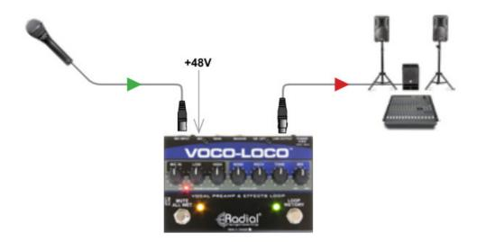
Connect the XLR output to a mic input on your PA system. The VocoLoco's output level will work equally wellwith a mic or line level input. If you hear distortion, lower the level on the Voco-Loco or reduce the sensitivity of the mixer's input channel.
