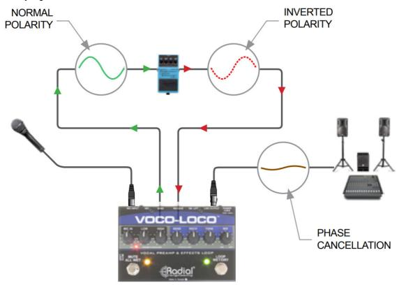
weak because an effect pedal is inverting it's output, compensate by pushing in the recessed 180° polarity reverse. This will invert the wet signal and bring it into phase with the dry signal to create a full sound.
