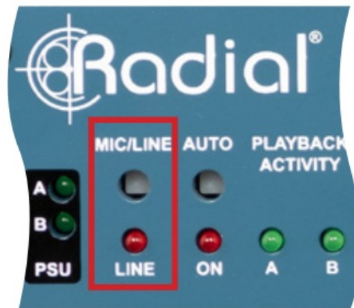
Front panel XLR MIC/LINE switch
