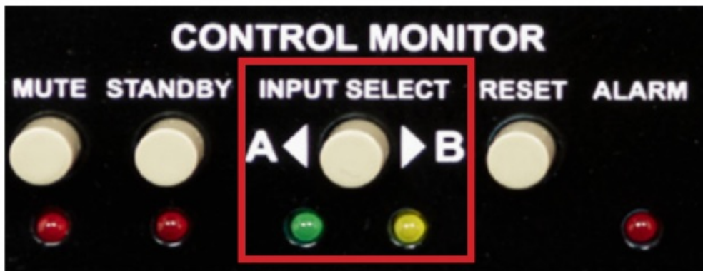
The INPUT SELECT switch on the front panel
