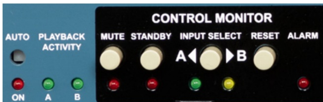
The AUTO-SWITCH controls on the SW8-USB
