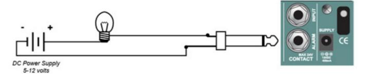
Normally, the relay is in an 'open' state preventing current from flowing through the external circuit. If the drone signal feeding the AUTOGATE input falls below the set THRESHOLD level, the relay closes allowing current to flow through the external alarm circuit and the front panel ALARM LED illuminates. When the drone track is restored the relay opens and the alarm turns off.
