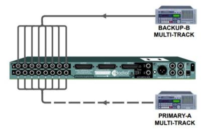
Primary and backup multi-tracks connected to the D-Sub inputs.
