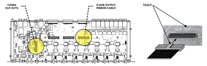
Shown in the default configuration with a direct line-level D-Sub output.
