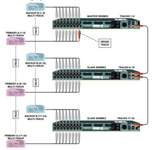
When combining two SW8 MK2 (second generation) units together, make sure the LINK-MODE switch on the top panel is set to the SW8 MK2 position. When combining your second generation SW8 MK2 with a first generation SW8 MK1, the switch needs to be set to the SW8 MK1 position. This ensures that both units switch in proper sync.
