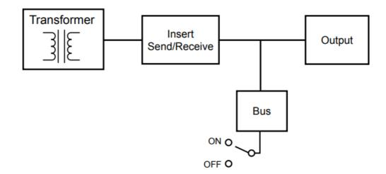
• When using the Space Heater as an effect on individual channels, the insert jacks can be used as a patch bay. This can be convenient for connecting other pieces of equipment to your signal chain while already in the analog domain, or to simply use the insert "SEND" jack as a parallel output for recording or processing elsewhere. Keep in mind that the insert jacks are still the last step in the Space Heater's signal path, so any equipment inserted will be processing the wet sound.
