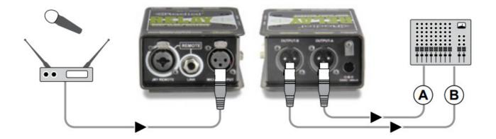
Switching between the outputs can be done using the OUTPUT SELECT push button on the side panel. Start by setting up channel-A. Set the AB selector switch set to the A position (outward). Speak into the mic while slowly bringing up the volume levels. To set up the channel-B depress the AB selector switch to toggle the output. The LED indicators illuminate to display the active output.
