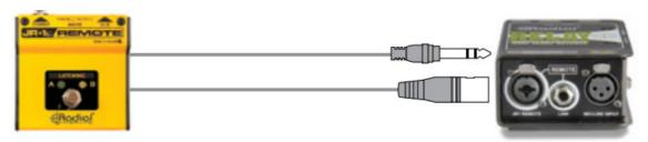
The JR1 uses either 1/4" or locking XLR cable to connect to the Relay Xo.
