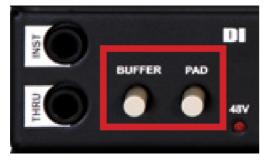
Note that if you have an instrument with active pickups, or if you use buffered guitar pedals anywhere in the signal chain, this switch will likely have no audible effect. Wait 60 seconds after powering the D.I. with 48V before activating the BUFFER switch, as it takes a short amount of time to charge before it is ready for use.
