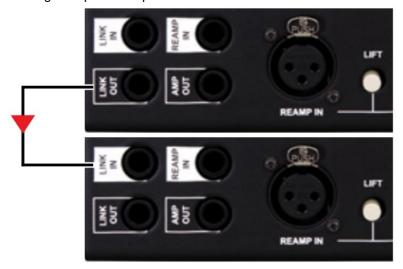
The LINK OUT carries a copy of the same balanced signal that you feed to the input of the Reamper, and it won't be affected by any of the controls on the Reamp Station. If your audio interface is short on linelevel outputs, you can use this feature to feed a compressor on another outboard effects processor at the same time that you are Reamping with the Reamp Station.
