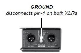
The second ground lift is simply labeled LIFT and is located on the input panel. This switch allows the right channel ground to be lifted separately from the left channel and is intended for dual mono applications where one source device needs a ground path through the ProAV2 while the other may not. Note that the GROUND switch supersedes the LIFT switch and disconnects the ground path for both channels regardless of the position of the LIFT switch.
