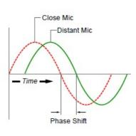
This minute delay creates a phase shift between the two mic signals that colors the tone through a type of phase cancellation known as comb-filtering. The Phazer exploits this phenomenon and presents it as a simple, fun and musical tool for the audio engineer.
