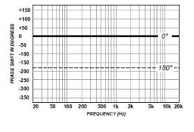
Bypass - zero phase shift, response is linear.
