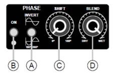
For the most part the goal is to shift the close mic signal until the fundamentals phase-align with the distant mic in a musical and pleasing way that compliments the instrument and program material. Keep in mind it is impossible for all frequencies to line up or be in perfect phase at the same time. When tuning the SHIFT control, simply use your ears to find what sounds best to you.
