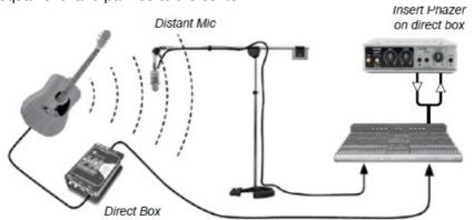
Once you have the D.I. and mic set up take a look at the time line below. It will help you understand what you are hearing. When the guitar is strummed the D.I. sends an electronic signal at nearly the speed of light while the mic has to wait for the slower sound waves to travel through the air. This creates a phase shift between the two
