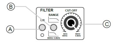
Slowly turn the CUT-OFF control counter-clockwise while listening to the effect. As you turn the CUT-OFF control counter-clockwise the filter moves downward through the spectrum removing frequencies above the cut-off point from the Phazer's output.
