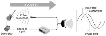
So, how does it sound? What you are hearing is the complex interaction between the DI, mic and the room causing phase cancellations at some
