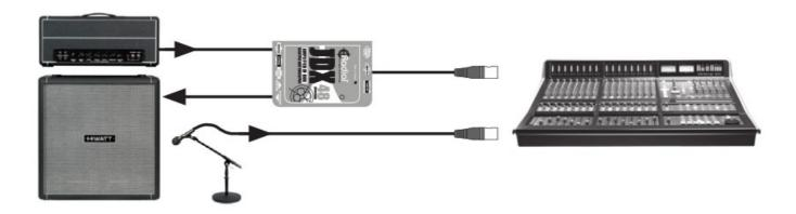
Using the JDX 48 with the Radial Phazer: When the signal from the JDX 48 and a microphone combine there will inevitably be a small time delay between the signals. The Radial Phazer can be used to time-align the JDX 48 signal with the microphone for fat sounds and effects.
