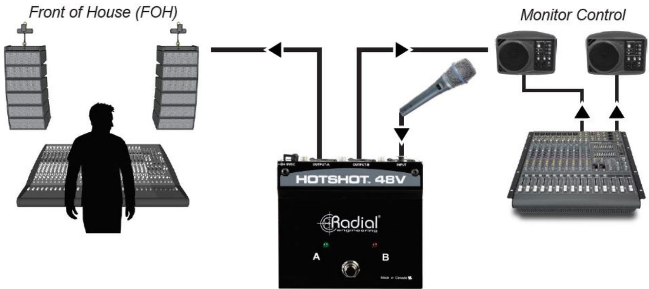
The HotShot 48V makes it easy to switch signals between FOH and Monitors on stage.
