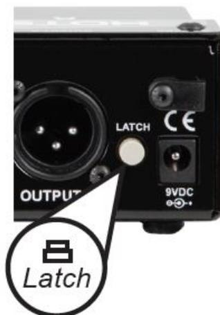
This switch can also be configured for latching operation. To do so, press the LATCH switch on the rear panel. In this mode a single press of the Toggle footswitch will switch the microphone to Output-B, requiring a second press of the footswitch to switch back to Output-A.
