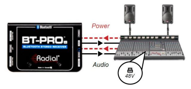
Powering the BT-Pro using 48V phantom power
