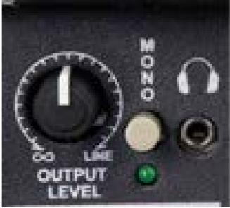
Adjusting the level control on the BT-Pro will affect both the XLR and headphone output. The intended use of the headphone output is for testing purposes to ensure that signal is being properly received by the BT-Pro. If you do not hear sound in the PA, signal present at the headphone output lets you know that the problem is likely not the BT-Pro but maybe another connection or that a piece of equipment needs to be checked.
