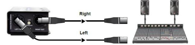
Audio connections for PA system and recording systems use balanced XLR cables up to 100 meters (300').
