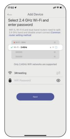
• Follow the guide on the APP to press and hold the button on the mini box hub for about 5 seconds until the connecting indicator quickly blinks.
