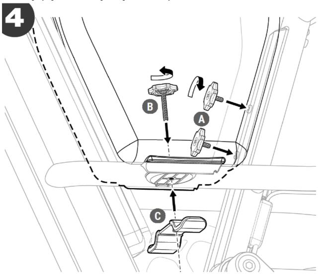
5. Console fully installed. Note the position of the mounting bracket (C).
