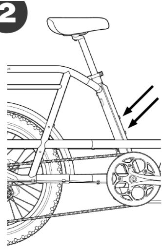
3. Press the tabs (see bottom arrow) on either side of the top half's interior to allow the tabs to slide through the slots. Then you can lift off the top.
