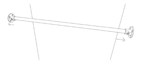
Mount with screws and plugs. Fasten pipe with key clamp.
