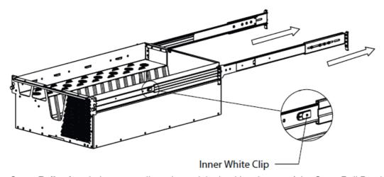
2. **Attach the Outer Rails**: Attach the outer rails to the rack by hooking the top of the Outer Rail Bracket into the top hole of the "U" space. Secure the rails by installing (1) Truss Head Screw per side into the Outer Rail Brackets. Install the rst set of rails loosely and the second set of rails tightly.
