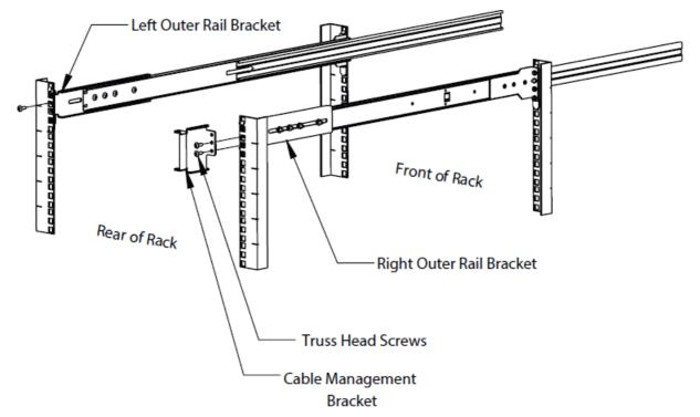
4. **Install the HyperShelf:** Slide the shelf into the Outer Rails. Pull the blue tab on the inner rail to slide all the way in. Screw in the Thumb Screws to secure in place. Tighten loose rails to ensure that the HyperShelf slides into both rails at the same time. Two people are recommended for installation
