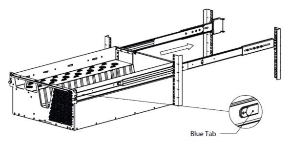
5. Install the Cable Management Arm: Attach the Cable Management Arm to the HyperShelf by putting the Cotter Pins through the Cable Management Brackets attached to the shelf and to the Outer Rail. For detailed information on installing the Cable Management Arm, follow the instructions included in the Cable Management Arm box.
