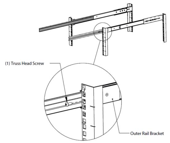
3. **Secure the Rear Outer Rails**: Secure the rear of the outer rails by installing the (1) Truss Head Screw into the left Outer Rail Bracket, and install the (2) Truss Head Screws through the Cable Management Bracket and into the right Outer Rail Bracket.
