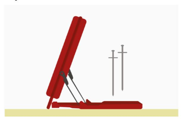
The mount can also be used as a stand with the Track Box standing on the ground angled upwards. On soft/uneven ground it may be necessary to use the supplied stakes to secure the Track Box in position, these can be pushed slotted through the stake holes and then pushed into the ground.
