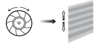
Rotate the scroll wheel to incrementally raise or lower the shade. For other operations, please refer to the motor operation instructions.
