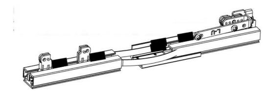
**Step 2.** Remove all packaging material from the Track, ensuring the Drive Belt stays in place inside the Track.
