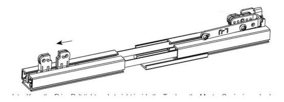
**Step 4.** Bring both Master Carrier Body halves together and insert the center clip.
