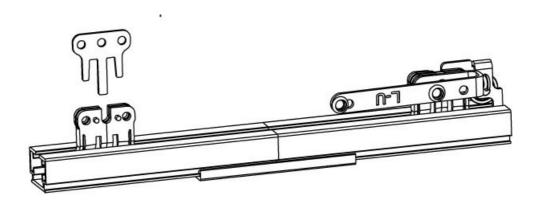
Step 5. Tighten the Splice set screws.
