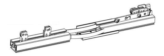
**Step 3.** Bring the Track sections together by pushing the Track onto the Splice and moving the Master Carrier forward.
