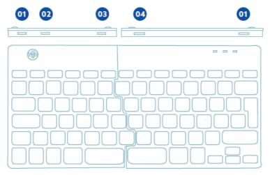
• A. Connect the two parts by plugging cables 02 or 03 into ports 03 and 04.
