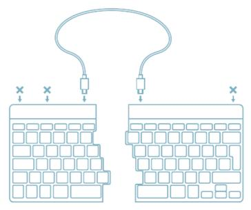
• **B.** Connect the keyboard to your computer by plugging the USB-C end of cable 01 into port 02 and the other end into the USB port of your computer.
