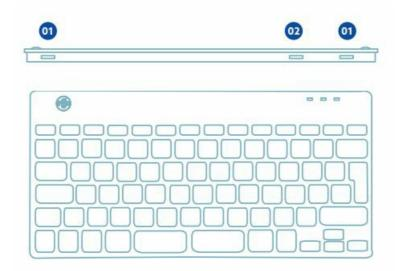
Connect the keyboard to your computer by plugging the USB-C end of cable 01 into port 02 and USB-C end into your computer.
