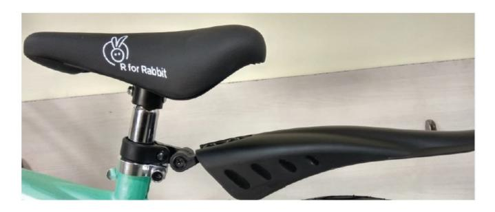
Insert the saddle tube vertically into the frame riser below the safety line of 65mm. Safety line should not be exposed. Adjust the seat to the appropriate height and then the fasten the saddle screws. Adjust the height of back mudguard by loosening the screw.
