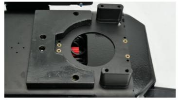
1. Thread four M3 screws into the screw holes to lock the Q-DVL in place.
