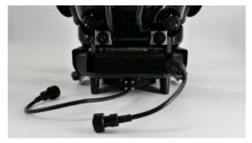
2. Please attach the connector of the Q-DVL to the A3 or A4 Q-interface only. Attach the connector of the side scan sonar to any Q-interface on the ROV.
