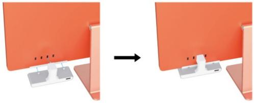
Step 2: Plug the USB-C hub into the Thunderbolt port on the rear of 2021 iMac.
