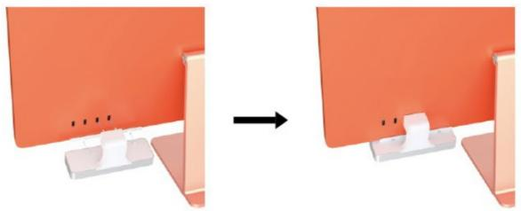
Step 2: Plug the USB-C hub into the two Thunderbolt ports on the rear of 2021 iMac.
