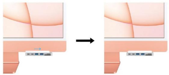
Step 3: Put the USB-C hub into the notches on the plastic fin and slide it to on the right.
