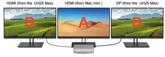
• When connecting HDMI (from Mac mini), HDMI (from the UH25 Max), and DP (from the UH25 Max) at the same time, it does support the extended mode of A-B-B. It does not support the extended mode of A-B-C.
