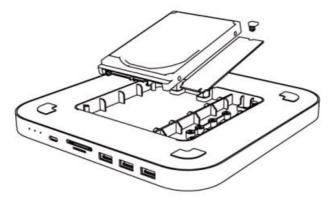
2. Insert a 2.5-inch SATA HDD or M.2 NVMe SSD into the slots.
