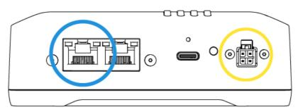
Before connecting  $P \square E$  to your router, please check specification of your model. Connecting  $P \square E$  to model that's not supporting  $P \square E$  con damage your router.
