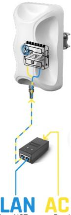
Please note that Semtech XR60 router does NOT support Passive PoE on the ETH port
