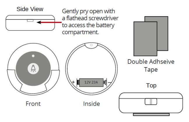
Place double adhesive tape on back of call button and mount to wall.
