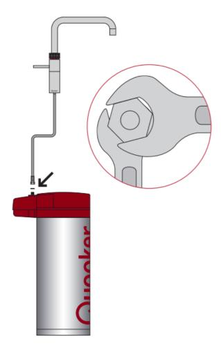
5. Connect the tank hose back onto the Inlet Reducing valve using the large blue fibre washer and spanner 22.
