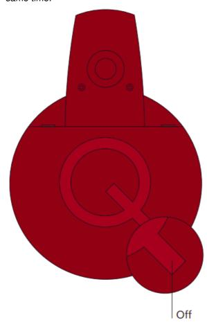
2. Close the Isolation Valve then run the boiling water tap again. If it is depressurised, no water will flow out of it.
