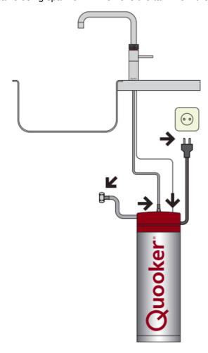
4. Place the new tank. Reconnect the tap hose to the top of the tank with the small washer using spanners 10/12 and 14.
