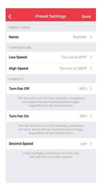
These settings will be saved into the memory of the Hub meaning all settings will sync between any additional devices you pair to the Hub.
