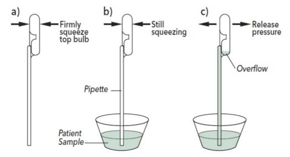
**Note:** The pipette is designed to collect and dispense the correct amount of liquid sample.
