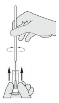
4. Place the Test Strip into the tube with the arrows pointing down. Do not handle or remove the Test Strep for 15 minutes.
