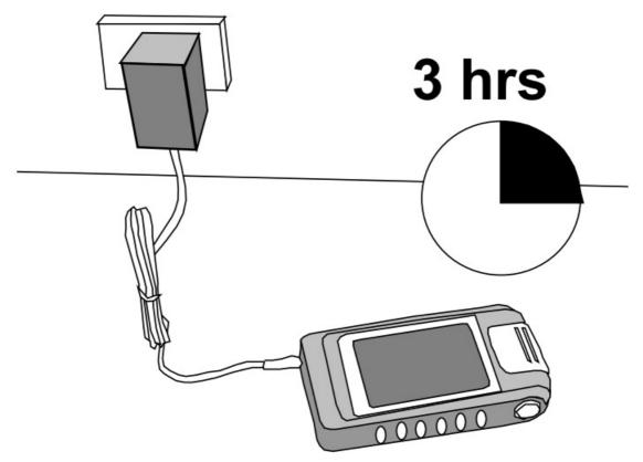
The red light beside the power connector should illuminate indicating that the battery is being charged. The light will go off when the battery is substantially charged. It takes about three hours to charge the battery from a discharged state. Quicklook Touch can be used while the battery is being charged.
