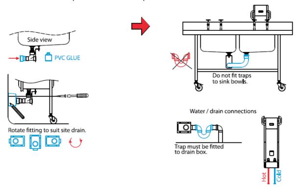
Ensure all pipework is flushed clear of debris. Service valves should be fitted to supplies. Max. recommended water pressure 3 bar (44psi) Earth bonding connection required. Installation must comply with local authority requirements.
