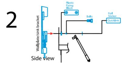
3. Level wall plate. fix top 2 wallplate fixings to wall.
