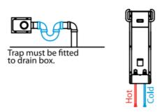
Ensure all pipework is flushed clear of debris. Service valves should be fitted to supplies. Max. recommended water pressure 3 bar (44psi) Earth bonding connection required. Installation must comply with local authority requirements.
