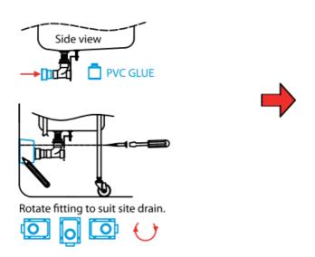
9. Interconnect drains into open and of tee or cap
