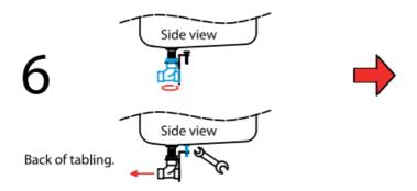
Tighten buffer against underside of bowl Lock in place.
