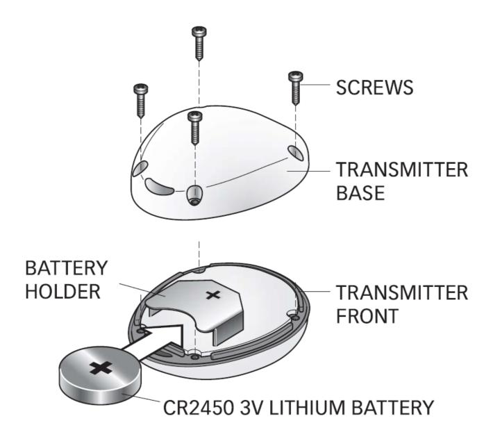
**WARNING**: once the transmitter is assembled, verify that the LED does not remain on constantly. If the LED is on, reopen the transmitter and verify that it was assembled correctly.
